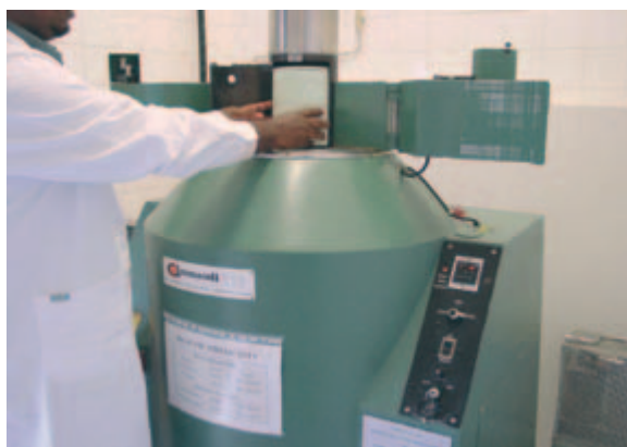
FIG. 9. Self-contained dry-storage gamma irradiator suitable for research and small-scale irradiations. In preparation for irradiation, a sample holder is being placed in the irradiation chamber when it is in the loading position. Depending on the dose rate of the day, the timer on the control panel (bottom right) is set to give the desired dose.
