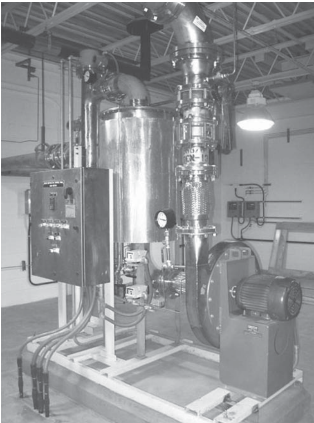
Figure 15.27. Ozone destruction unit.
