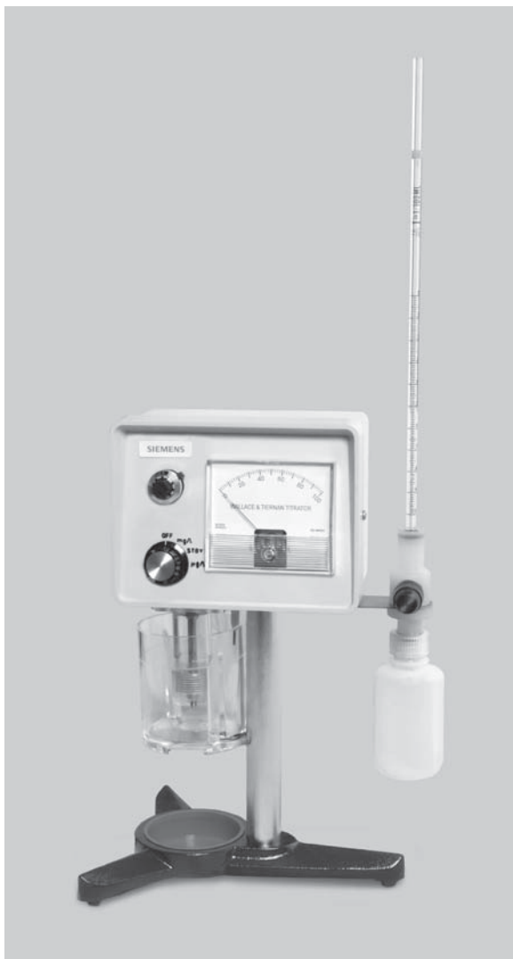
Figure 3.1. Amperometric titrator (courtesy of Siemens Water Technologies).
