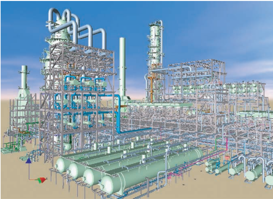
Figure 8.1 3D laser scan “as-built” software modeling (examples courtesy of INOVx Solutions, Irvine, California).
