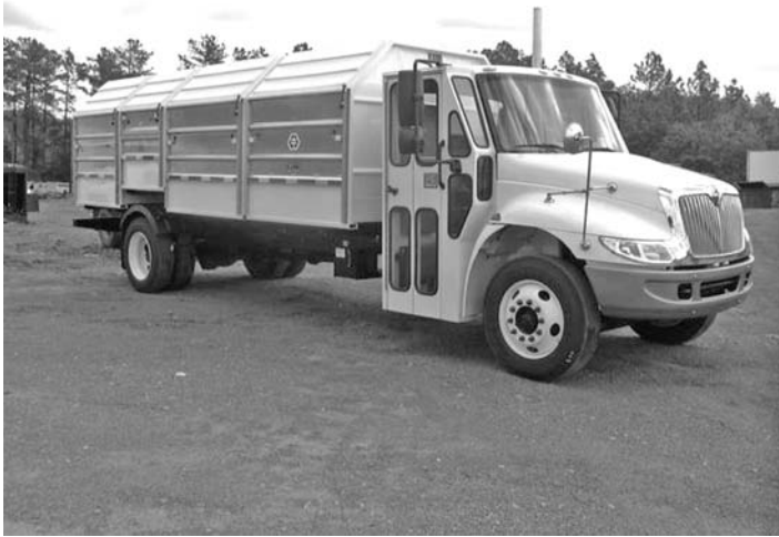
FIGURE 3.4 Sorting truck for unseparated recyclables. (From Kann Manufacturing Corp., http://www.kannmfg.com/curbsorter.htm . With permission.)
