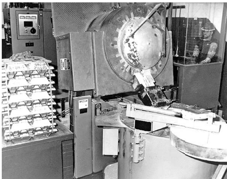
FIGURE 14.2 An operator-shielded melt control station for furnace charging. (From Inductotherm, Inc., Safety Manual, http://www.inductotherm.com/safety/safety.htm , n.d. With permission.)
