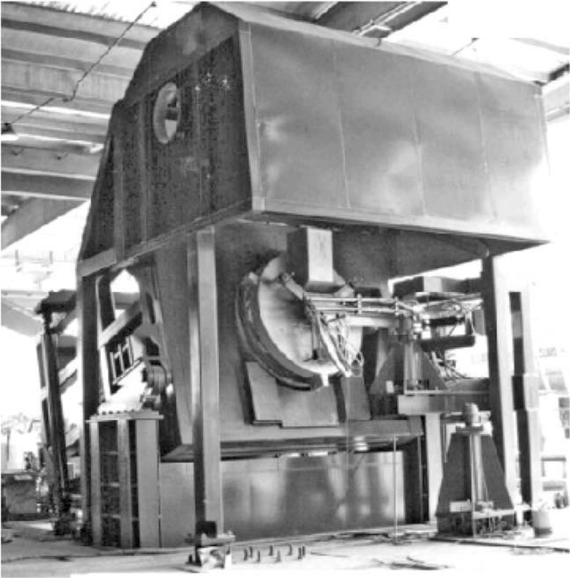
FIGURE 9.9 View of a rotary melting furnace. (From MDY Engineering, http://www.mdy-engineering.com/images/VCM_14_MT_2.jpg . With permission.)
