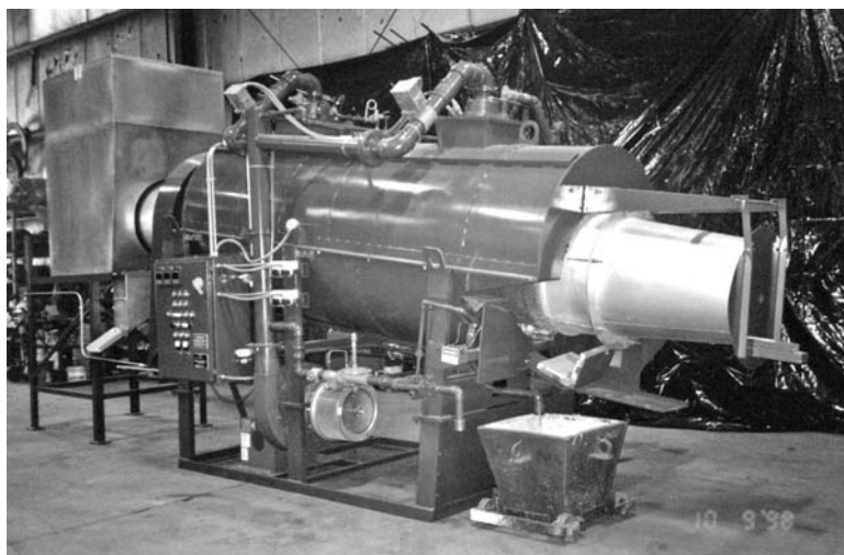
FIGURE 5.26 A large-scale rotary sweat furnace. (From EnviroAir, Inc., http://www.enviroair.net/RotarySweatFurnacePage.htm . With permission.)
