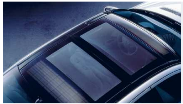
Micro-structured solar cells integrated in car sunroofs could be substituted by nano solar cells in future [© DaimlerChrysler AG]
