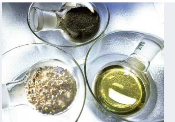
Tyre components: Soot (carbon black) above, Silica bottom left and Organosilane bottom right [© Degussa AG]
