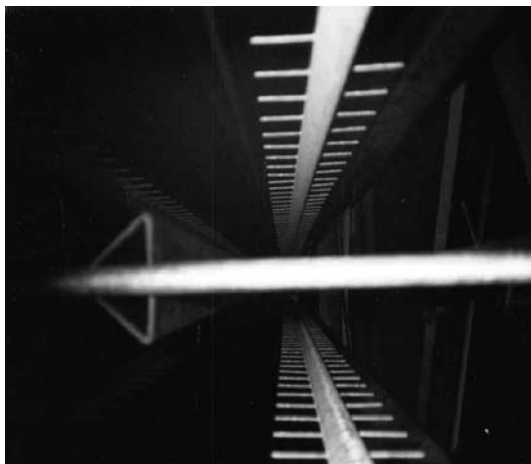
FIGURE 18.13 Discharge electrode and G-Opzel collecting plate. (With permission from Hamon.)
