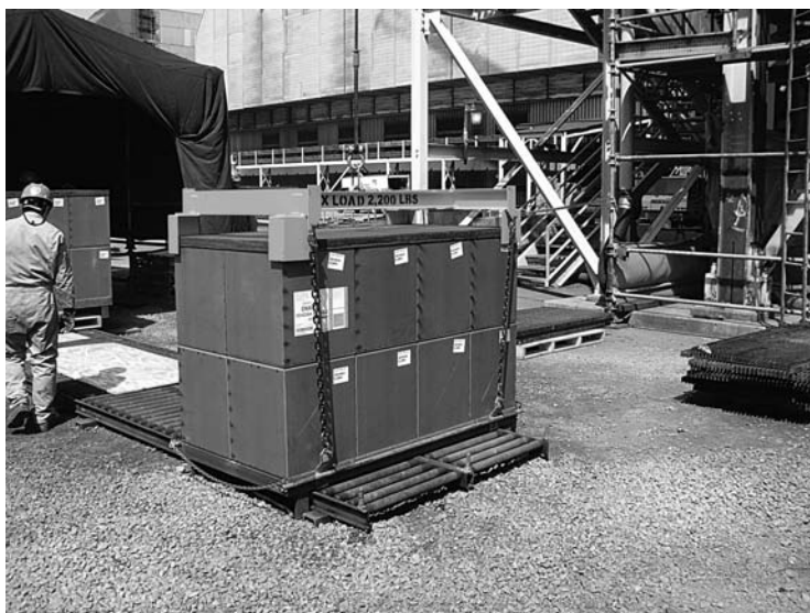
FIGURE 17.16 SCR catalyst module for high particulate flue gas service. (With permission from Haldor-Topsoe, Inc.)
