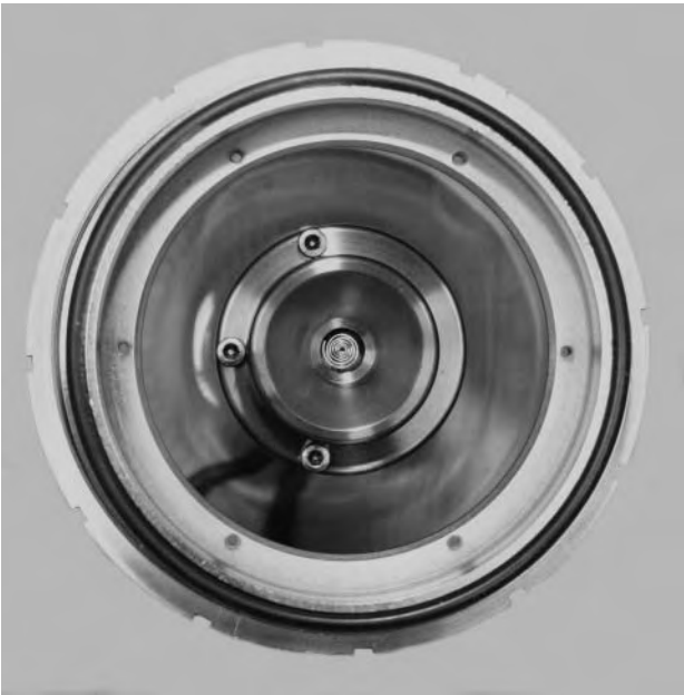
FIGURE 11.10 Cathode assembly from an Elekta SL series linac. Note the spiral cathode at the centre.
