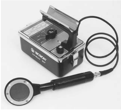
Fig. 12-10 Geiger counter with a thin “beta window.”
