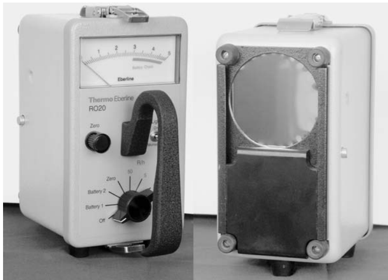
Fig. 12-12 Portable ion chamber instrument with a removable beta shield cap.
