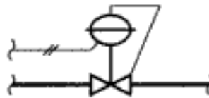
FIGURE 2-51 Double-acting diaphragm operator.
