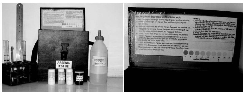
Figure 1 Colorimetric field test kits with corresponding colored scale chart. (See insert for color representation of figure.)
