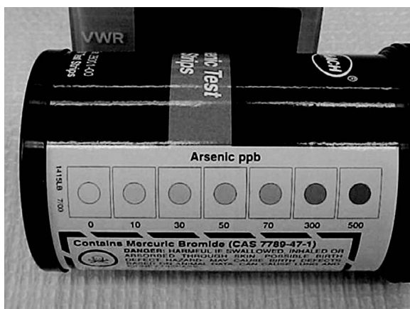
Figure 2 Container for bromide strips showing printed color chart corresponding to solutions containing 0, 10, 30, 50, 70, 300, and 500 \mu\text{g/L} of arsenic. (From ref. 9.) (See insert for color representation of figure.)
