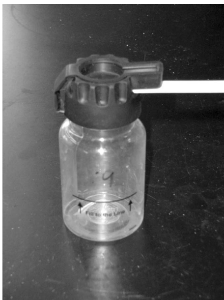
Figure 1 Reaction vessel with test strip in place. The graduated mark indicates the level corresponding to 50 mL of sample solution. (From ref. 9.)
