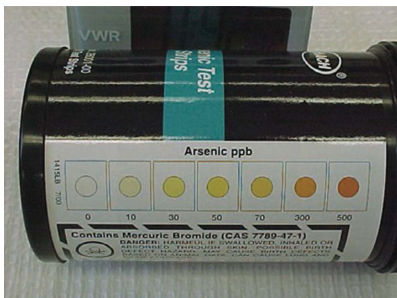
Chapter 7, Figure 2 Container for bromide strips showing printed color chart corresponding to solutions 0, 10, 30, 50, 70, 300, and 500 \mu\text{g/L} of arsenic.
