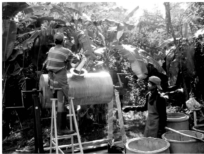
Figure 6 Batch reactor employed to carry out regeneration at the central regeneration facility. (See insert for color representation of figure.)
