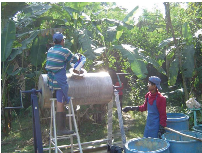
Chapter 13, Figure 6 Batch reactor employed to carry out regeneration at the central regeneration facility.
