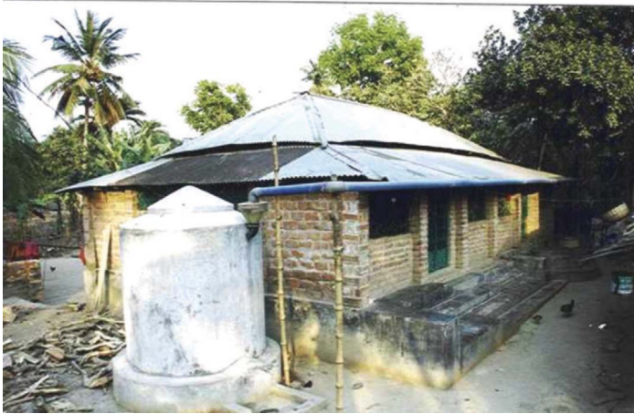
Chapter 14, Figure 6 Rainwater harvesting by roof catchment.
