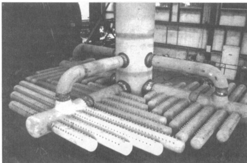
Figure 4-51. Air distributor—"pipe grid" design version. (Source: Enpro Systems, Channelview, Texas.)
