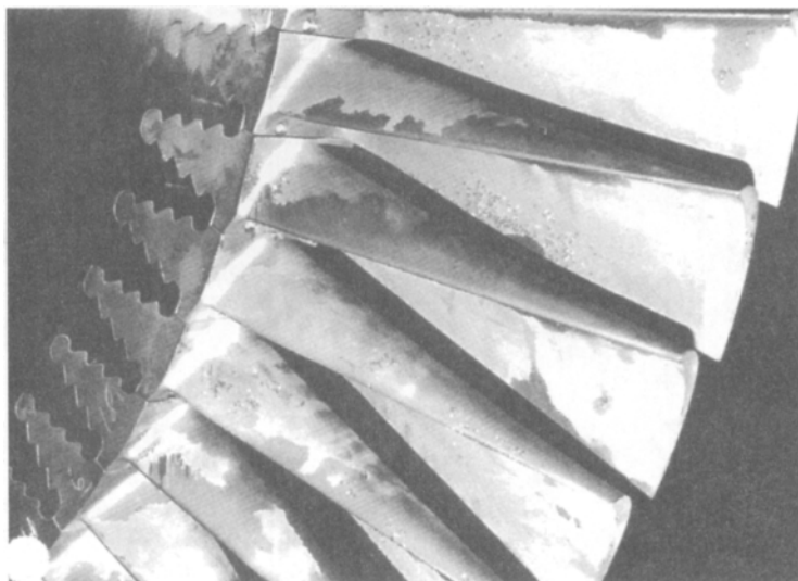
Figure 5-21. This picture shows the rotor blades from the inlet end. Root design is a four-land fir-tree type. A lock pin on each root platform locates the blade axially in the disc.
