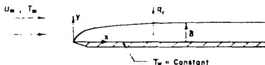
FIG. 9. Physical model and coordinate system for boundary layer flow of an absorbing gas.
