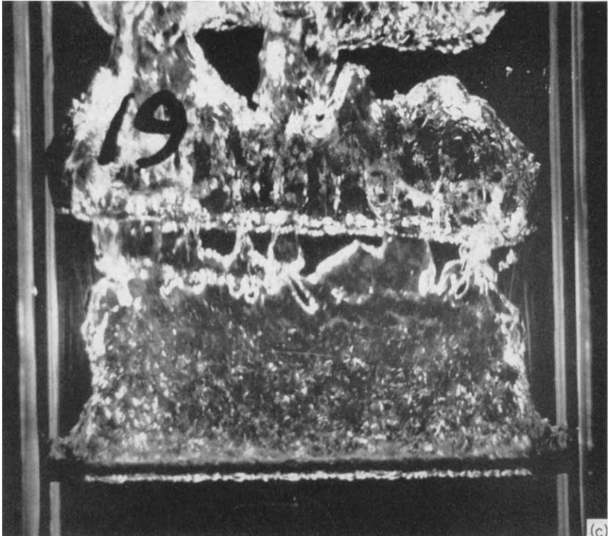
FIG. 27. Effect of heat flux on the boiling pattern of nearly saturated water (4° F subcooling) from a \frac{3}{16} -inch tube at 2 ft/sec (90). (a) 21% of critical flux. (b) 47% of critical flux. (c) 84% of critical flux.
